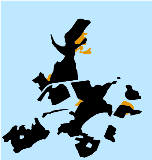
Abbildung 29: Wetland-Groundtruth in schwarz, True Negative Pixel in blau, False Positive in orange
